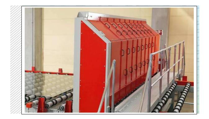
With 95% the float glass process is actually dominating he production of flat glass used for house windows, are windows, mirrors etc. Excellent Quality is very important for all different applications of glass in downstream operations. The float glass runs on the conveyor through the camera inspection system IQLine G, which detects all typical float glass defects.
