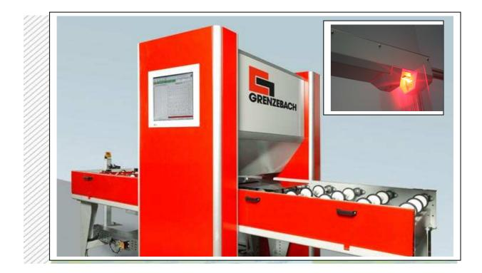
Leaving cutting lines glass panels have to be inspected especially for their right sizes, rectangularity and edge damages. Furthermore there might be grinding lines and other process steps which require inspection. Grinding defects are mostly inaccurate C- or K-shapes, shiners, burns and edge chips. Also additional handling scratches will be detected by using our Cutted Glass inspection solutions. The systems cover high production speeds, acceleration and deceleration of the glass panels
